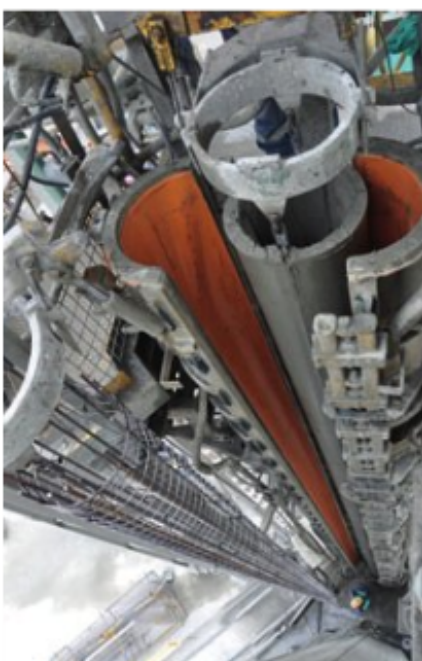
Fig. 2,3 and 4: De-moulding process of fresh poured poles.
