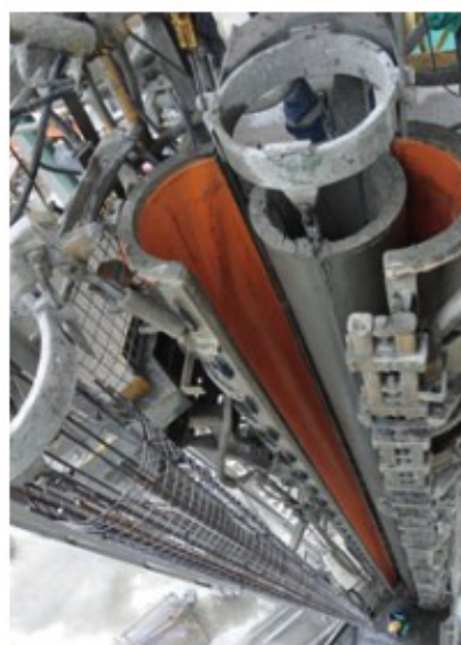
Fig. 2,3 and 4: De-moulding process of fresh poured poles.
